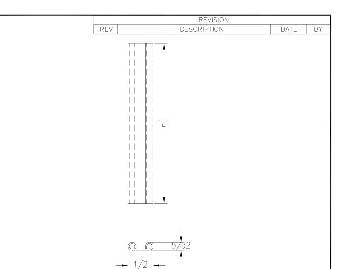
SEE PO FOR MATERIAL TYPE AND FINISH FOR LENGTH DIMENSION ("L"), SEE PURCHASE ORDER. LENGTH TOLERANCE:LESS THAN 60": ±1/16" LESS THAN 120": ±1/8", 120" OR GREATER: ± 1/4" MAXIMUM BURR NOT TO EXCEED 10% OF MAT'L THICKNESS WITH THE EXCEPTION OF CUT ENDS, WHICH MAY HAVE BURR EXCEEDING THIS AMOUNT. FINISHED PART MAY EXHIBIT TYPICAL ROLL FORMED END FLARE UP TO THREE INCHES FROM ENDS. PROFILE DIMENSIONS TO BE MEASURED 3" OR GREATER FROM CUT ENDS.
