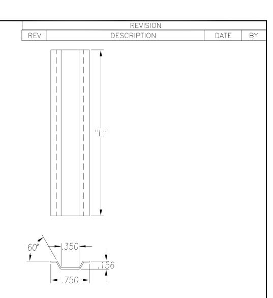
SEE PO FOR MATERIAL TYPE AND FINISH FOR LENGTH DIMENSION ("L"), SEE PURCHASE ORDER. LENGTH TOLERANCE:LESS THAN 60":  $\pm 1/16$ " LESS THAN 120":  $\pm 1/8$ ", 120" OR GREATER:  $\pm 1/4$ " MAXIMUM BURR NOT TO EXCEED 10% OF MAT'L THICKNESS WITH THE EXCEPTION OF CUT ENDS, WHICH MAY HAVE BURR EXCEEDING THIS AMOUNT. FINISHED PART MAY EXHIBIT TYPICAL ROLL FORMED END FLARE UP TO THREE INCHES FROM ENDS. PROFILE DIMENSIONS TO BE MEASURED 3" OR GREATER FROM CUT ENDS.
