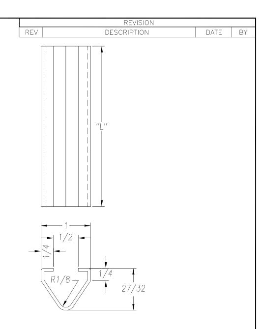
SEE PO FOR MATERIAL TYPE AND FINISH FOR LENGTH DIMENSION ("L"), SEE PURCHASE ORDER. LENGTH TOLERANCE:LESS THAN 60":  $\pm 1/16$ " LESS THAN 120":  $\pm 1/8$ ", 120" OR GREATER:  $\pm 1/4$ " MAXIMUM BURR NOT TO EXCEED 10% OF MAT'L THICKNESS WITH THE EXCEPTION OF CUT ENDS, WHICH MAY HAVE BURR EXCEEDING THIS AMOUNT. FINISHED PART MAY EXHIBIT TYPICAL ROLL FORMED END FLARE UP TO THREE INCHES FROM ENDS. PROFILE DIMENSIONS TO BE MEASURED 3" OR GREATER FROM CUT ENDS.
