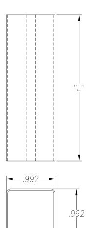
SEE PURCHASE ORDER FOR MATERIAL TYPE AND FINISH FOR LENGTH DIMENSION ("L"), SEE PURCHASE ORDER. LENGTH TOLERANCE: LESS THAN 60":  $\pm 1/16$ , LESS THAN 120":  $\pm 1/8$ ", 120" OR GREATER:  $\pm 1/4$ " MAXIMUM BURR NOT TO EXCEED 10% OF MAT'L THICKNESS WITH THE EXCEPTION OF CUT ENDS, WHICH MAY HAVE BURR EXCEEDING THIS AMOUNT. PROFILE DIMENSIONS TO BE MEASURED 3" OR GREATER FROM CUT ENDS.
