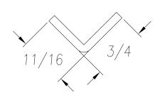
SEE PO FOR MATERIAL TYPE AND FINISH FOR LENGTH DIMENSION ("L"), SEE PURCHASE ORDER. LENGTH TOLERANCE:LESS THAN 60":  $\pm 1/16$ " LESS THAN 120":  $\pm 1/8$ ", 120" OR GREATER:  $\pm 1/4$ " MAXIMUM BURR NOT TO EXCEED 10% OF MAT'L THICKNESS WITH THE EXCEPTION OF CUT ENDS, WHICH MAY HAVE BURR EXCEEDING THIS AMOUNT. FINISHED PART MAY EXHIBIT TYPICAL ROLL FORMED END FLARE UP TO THREE INCHES FROM ENDS. PROFILE DIMENSIONS TO BE MEASURED 3" OR GREATER FROM CUT ENDS.
