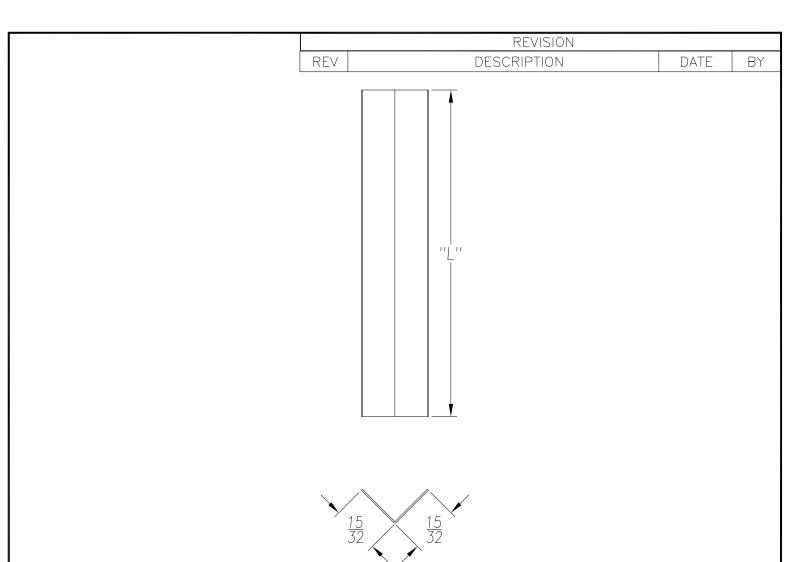
SEE PO FOR MATERIAL TYPE AND FINISH FOR LENGTH DIMENSION ("L"), SEE PURCHASE ORDER. LENGTH TOLERANCE:LESS THAN 60": ±1/16" LESS THAN 120": ±1/8", 120" OR GREATER: ± 1/4" MAXIMUM BURR NOT TO EXCEED 10% OF MAT'L THICKNESS WITH THE EXCEPTION OF CUT ENDS, WHICH MAY HAVE BURR EXCEEDING THIS AMOUNT. FINISHED PART MAY EXHIBIT TYPICAL ROLL FORMED END FLARE UP TO THREE INCHES FROM ENDS. PROFILE DIMENSIONS TO BE MEASURED 3" OR GREATER FROM CUT ENDS.
