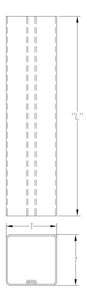
FOR LENGTH DIMENSION ("L"), SEE PURCHASE ORDER. LENGTH TOLERANCE:LESS THAN 60":  $\pm 1/16$ ", LESS THAN 120":  $\pm 1/8$ ", 120" OR GREATER:  $\pm 1/4$ " MAXIMUM BURR NOT TO EXCEED 10% OF MAT'L THICKNESS WITH THE EXCEPTION OF CUT ENDS, WHICH MAY HAVE BURR EXCEEDING THIS AMOUNT.
