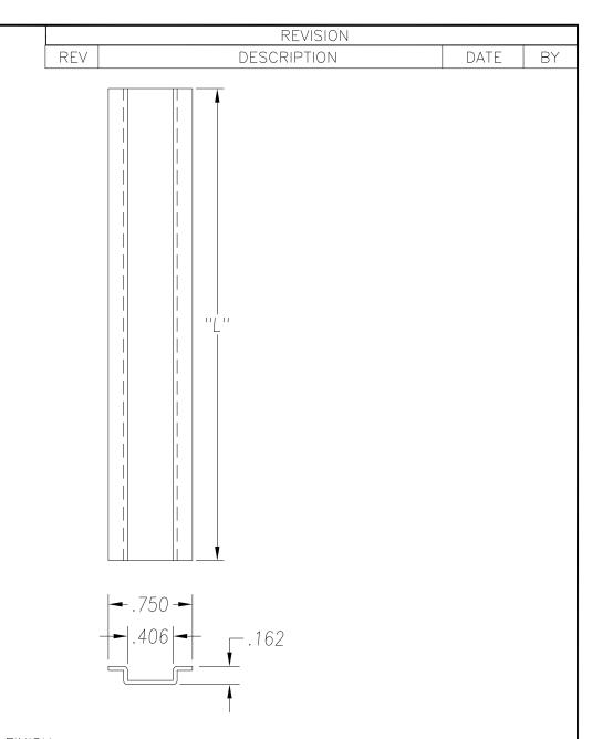
SEE PO FOR MATERIAL TYPE AND FINISH FOR LENGTH DIMENSION ("L"), SEE PURCHASE ORDER. LENGTH TOLERANCE:LESS THAN 60": ±1/16" LESS THAN 120": ±1/8", 120" OR GREATER: ± 1/4" MAXIMUM BURR NOT TO EXCEED 10% OF MAT'L THICKNESS WITH THE EXCEPTION OF CUT ENDS, WHICH MAY HAVE BURR EXCEEDING THIS AMOUNT. FINISHED PART MAY EXHIBIT TYPICAL ROLL FORMED END FLARE UP TO THREE INCHES FROM ENDS. PROFILE DIMENSIONS TO BE MEASURED 3" OR GREATER FROM CUT ENDS.
