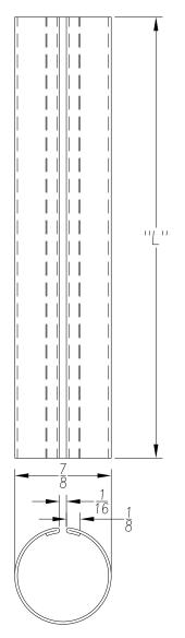
FOR LENGTH DIMENSION ("L"), SEE PURCHASE ORDER. LENGTH TOLERANCE: LESS THAN 120":  $\pm 1/8$ ", 120" OR GREATER:  $\pm 1/4$ " MAXIMUM BURR NOT TO EXCEED 10% OF MAT'L THICKNESS WITH THE EXCEPTION OF CUT ENDS, WHICH MAY HAVE BURR EXCEEDING THIS AMOUNT. FINISHED PART MAY EXHIBIT TYPICAL ROLL FORMED END FLARE UP TO THREE INCHES FROM END
