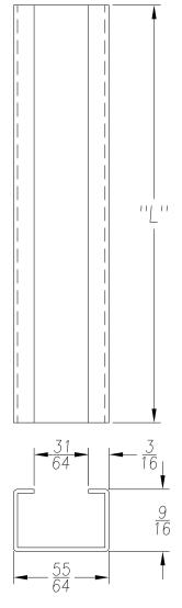
SEE PO FOR MATERIAL TYPE AND FINISH FOR LENGTH DIMENSION ("L"), SEE PURCHASE ORDER. LENGTH TOLERANCE:LESS THAN 60":  $\pm 1/16$ " LESS THAN 120":  $\pm 1/8$ ", 120" OR GREATER:  $\pm 1/4$ " MAXIMUM BURR NOT TO EXCEED 10% OF MAT'L THICKNESS WITH THE EXCEPTION OF CUT ENDS, WHICH MAY HAVE BURR EXCEEDING THIS AMOUNT. FINISHED PART MAY EXHIBIT TYPICAL ROLL FORMED END FLARE UP TO THREE INCHES FROM ENDS. PROFILE DIMENSIONS TO BE MEASURED 3" OR GREATER FROM CUT ENDS.
