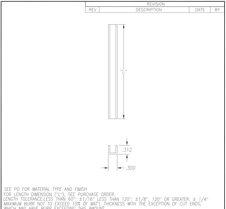
WHICH MAY HAVE BURR EXCEEDING THIS AMOUNT. FINISHED PART MAY EXHIBIT TYPICAL ROLL FORMED END FLARE UP TO THREE INCHES FROM ENDS. PROFILE DIMENSIONS TO BE MEASURED 3" OR GREATER FROM CUT ENDS.
